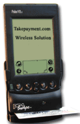
Figure 2 – Wireless PDA having a magnetic card reader incorporated
